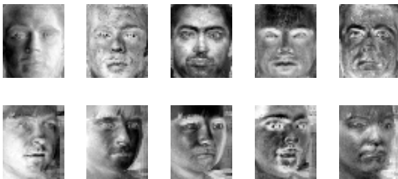
Figure 2: The first five eigenfaces (first to fifth from left to right) extracted by the standard PCA from the frontal (upper row) and half-profile (lower row) face images.
