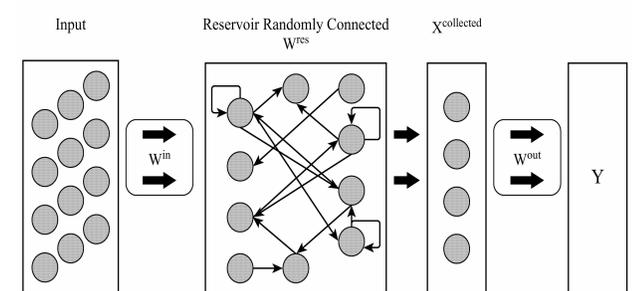
The structure of the ESN and readout system. On the left, the input signal is fed into the reservoir network through the fixed weights  $W^{in}$ . The reservoir network recodes these non-adaptively, and the output from the network is read out using the readout network weights  $W^{out}$ , which are learned.
