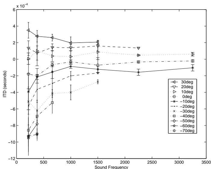
**Fig. 2.** Graph of ITD found for source angle between  $-70$  deg (i.e. left) and  $+30$  deg (right). Each line shows the ITDs found for stimuli of a particular frequency. Error bars are STDs of between 3 and 5 measurements. Results for low ITD (low angle) at lower frequencies have been omitted as they have a very high STD.
