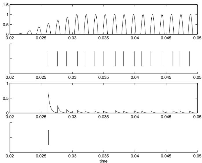
**Fig. 1.** Top shows 660Hz signal after cochlear filtering ( $F_c = 660Hz$ ) and rectification. Next line is the probabilistically generated spikes, followed by the depressing synapse EPSPs. Last line is the onset cell spike output. With above parameters, the onset cell fires on first input spike, but this is not crucial in this application.
