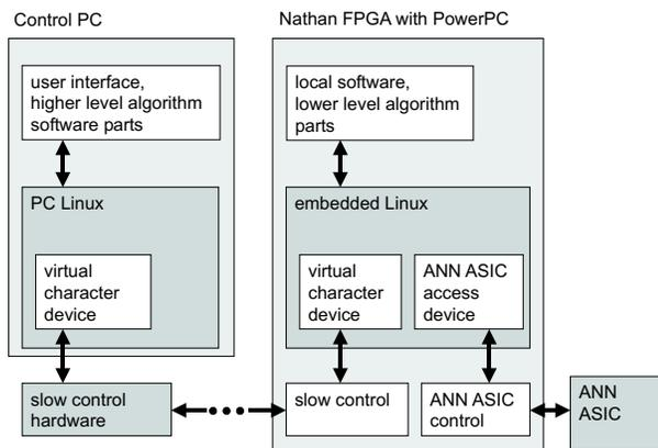
Fig. 5. Schematic view of software interaction between the controlling PC and one example PowerPC
