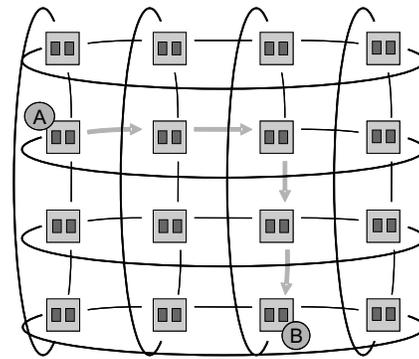
Fig. 4. The transport network forms a hardwired 2D-torus network on the backplane. During operation a worst case routing distance between two network modules *A* and *B* of four hops may occur.
