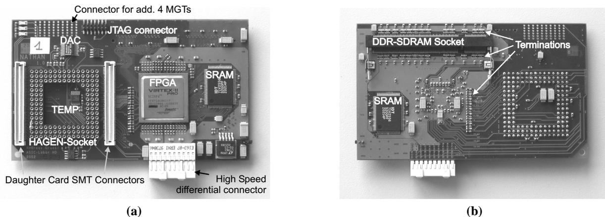
Fig. 3. Photographs of the presented network module. a) Top view. b) Bottom view.
