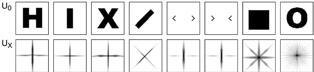
Figure 9: Axes of symmetry extracted from patterns having two or more axes.
