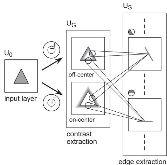
Figure 2: Extraction of oriented edges from positive and negative contrast components.
