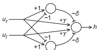
Figure 5: An example of a circuit calculating  $h = \gamma(u_r + u_l) - \delta|u_r - u_l|$ .
