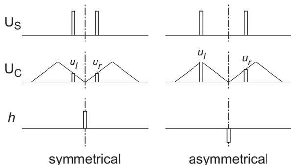
Figure 4: Illustration of the process of calculating  $h$ . When the stimulus is symmetrical,  $u_r = u_l$  holds. Hence,  $h$  takes a positive value. When the stimulus is asymmetrical, however,  $u_r$  and  $u_l$  take different values, and  $h$  becomes negative even though the values of  $u_r$  and  $u_l$  themselves are large.
