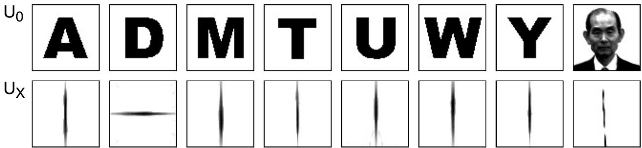
Figure 8: Axes of symmetry extracted from various input patterns.
