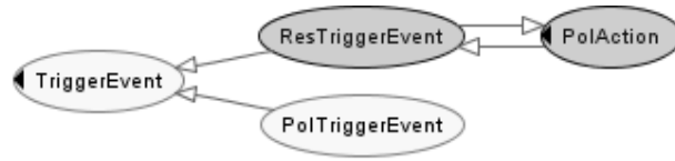
Figure 11. Resolution Policy Trigger Class Hierarchy
