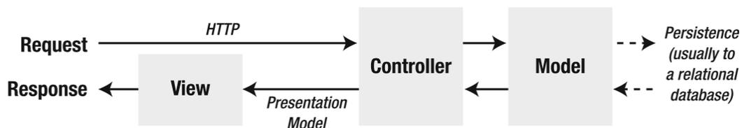
**Figure 16. The interactions in an MVC application**
