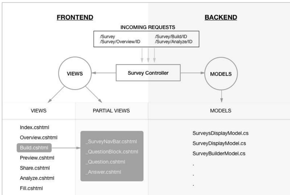
**Figure 27. MVC Project Structure**
