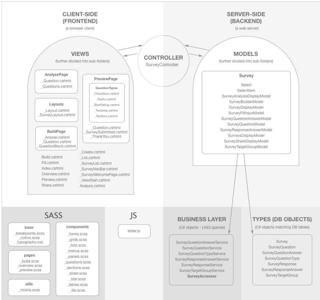
**Figure 29. The Final Project Structure**
