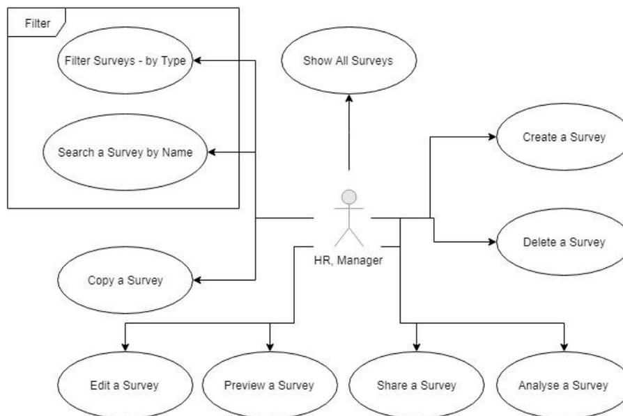
**Figure 21. HR and Manager Use Case Diagram**
