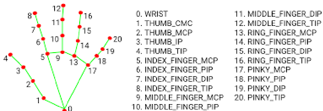
Figure 12: MediaPipe hand tracker provides 21 hand landmarks for innovative solutions
