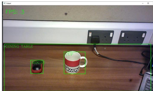
Figure 21: When SSD makes large object detections such as "Dining Table" the frame rate drops substantially
