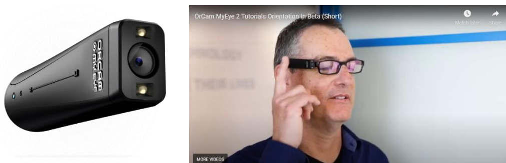
Figure 2: OrCam MyEye 2.0 magnetically attaches to a pair of glasses and is touch enabled
