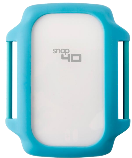
snap40 monitoring device The device is secured to the upper arm with an elastic arm band; allowing continuous monitoring of a patient.
