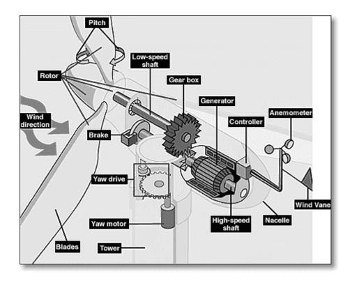
Figure 2.2: Wind Turbine Nacelle (Source: http://www1.eere.energy.gov)
