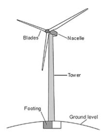
Figure 2.1: Wind Turbine Components (Source: http://www.seda.nsw.gov.au)
