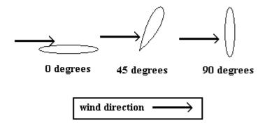
Figure A.1: Blade Pitch and Wind Direction
