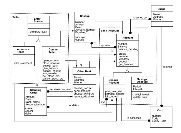
Figure 6.7: Refined object model
