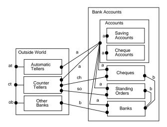
Figure 7.1: Class templates offering all their services in a single gate
