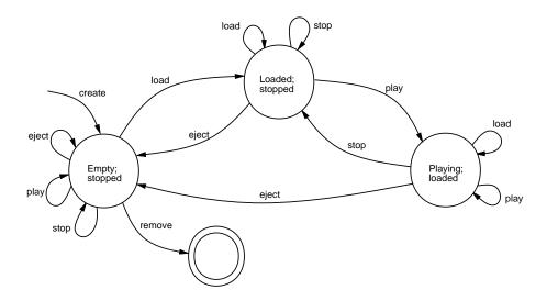
Figure 4.10: Behaviour of the video player example defined as a finite state automaton
