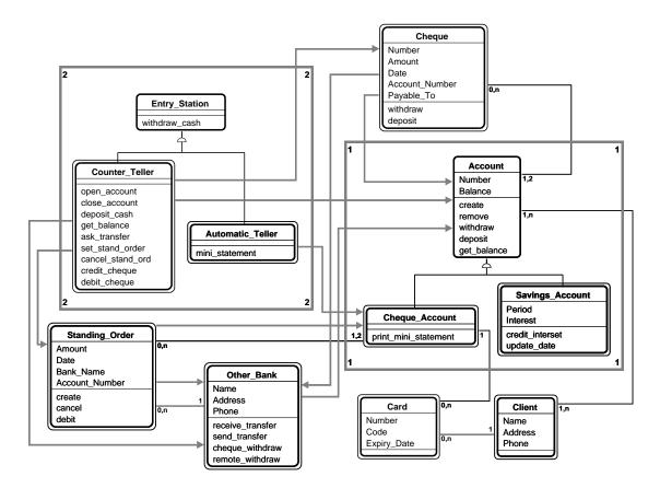
Figure 3.2: A Coad and Yourdon object model for the banking system
