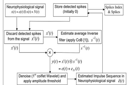
Fig. 4 Block diagram of iterative Cepstrum of Bispectrum based spike detection technique.
