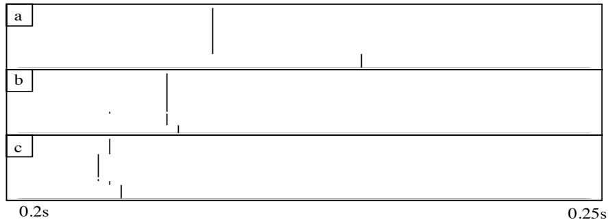
Figure 3: Results for a 50 ms section of the claps sound using the silicon neurons. (a) input attenuated to quarter original strength, dissipation = 10 (b) input attenuated to half original strength, dissipation = 20 (c) full strength input, dissipation = 40.
