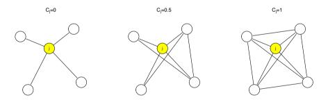
**Fig. 9.1** In the left image the clustering coefficient of node j,  $C_j = 0$  since there are no links among j's neighbors. In the middle image  $C_j = 0.5$  because three out of the possible six edges among the neighbors of j are present. In the right image  $C_j = 1$  as all the edges that could be there are actually present (it is a clique).
