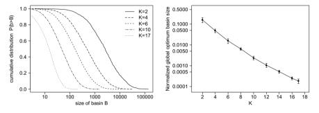
**Fig. 9.4** Size of the basins of attraction for *NK* Landscapes. **Left**: cumulative distribution of basin sizes for landscapes with N = 18, and selected values of *K*. **Right**: average normalized size of the basin of the global optimum. Averages (points) and standard deviation (bars) refer to 30 instances for each *K* value.
