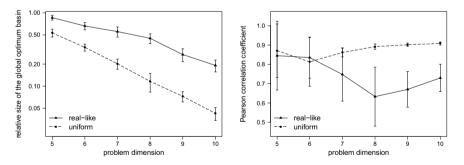
**Fig. 9.10** Basins of attraction in QAP instances. **Left**: Normalized size of the basin of the global optimum. **Right**: Pearson correlation coefficient between the fitness value of an optimum and the logarithmic size of its basin. Averages (points) and 0.95 confidence intervals (bars) are estimated with a t-test over 30 instances for each combination of problem class and size.
