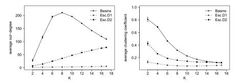
Fig. 9.6 Local connectivity for *NK* landscapes. Left: Average out-degree. Right: Average clustering coefficient. Averages (points) and 0.95 confidence intervals (bars) are estimated by a t-test over 30 random instances with N = 18.
