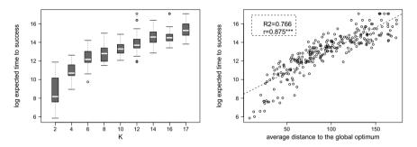
**Fig. 9.9** Performance of ILS on *NK* landscapes. **Left**: distribution of the expected running times to success for different *K* values. **Right**: correlation between the expected running times and the average shortest path to the global optimum. The regression line is dashed. The legend gives the ratio of variance explained by the regression, R2, and the Pearson correlation coefficient, *r*, with the asterisks indicating its significance level.
