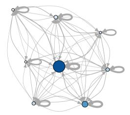
**Fig. 9.2** Local optima network with basin-transition edges for an *NK*-landscape instance with N = 18, K = 2. The size of the nodes is proportional to the basin sizes. The nodes' color represent the fitness values: the darker the color, the highest the fitness value. The edges' width scales with the transition probability (weight) between local optima.
