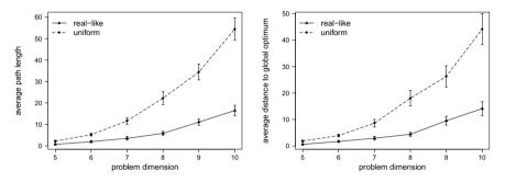
**Fig. 9.11** Shortest paths in QAP instances. **Left**: average path length. **Right**: average length of the shortest paths to the global optimum. Averages (points) and 0.95 confidence intervals (bars) are estimated with a t-test over 30 instances for each combination of problem class and size.
