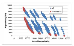
Figure 3. Exhaustive set of refurbishment options for one house in the synthetic example problem, with the Pareto optimal solutions highlighted.
