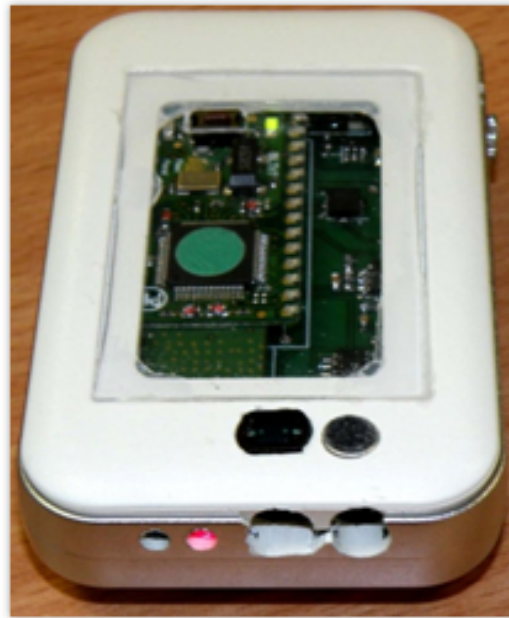
(b) Wearable Device for Recording Accelerometer, Light and Sound Data.
