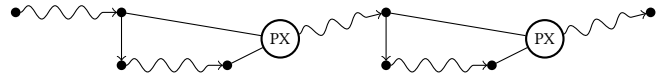
Figure 4: Graphical illustration of DRILS. Curly arrows represent HBHC while normal arrows represent a perturbation flipping \alpha N random bits.
